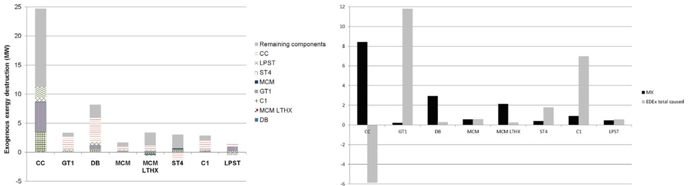
Figure 4. Defining the sources of exogenous rate of exergy destruction within each component (MW).
