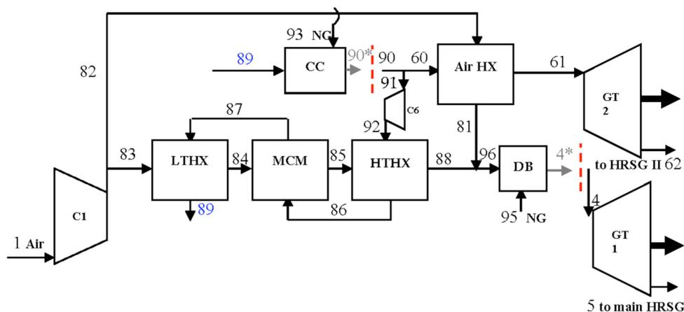
Figure 3. MCM reactor as part of the GT system of the AZEP 85 (Stream 89 exits the LTHX and enters the CC of the plant).
