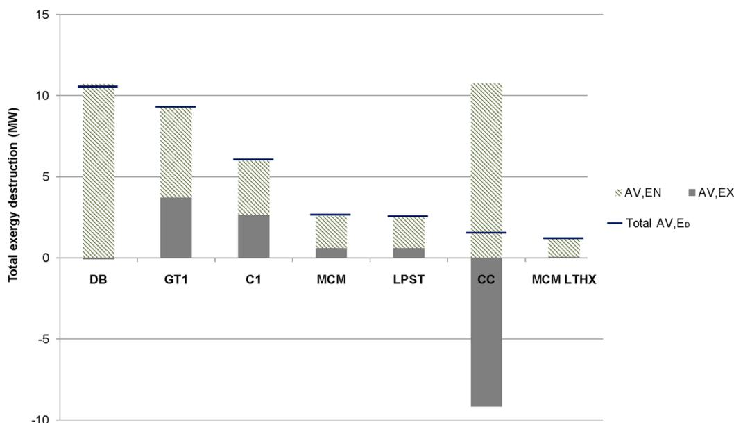
Figure 5. Total avoidable exergy destruction caused by each component (MW).
