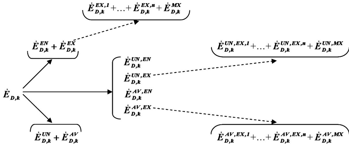
Figure 2. Options for splitting the exergy destruction in an advanced exergetic analysis.<sup>14</sup>
